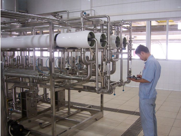
FIGURE 4.1 Picture of ultrafiltration membrane system for soy sauce processing.
